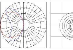
Maximum Candela=474.6 Located at Horizontal Angle=180, Vertical Angle=132.5
