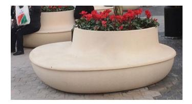
Jules et Jim are versatile ultra-high-performance concrete planters with bases that form a bench. Jim and Jules can live as separate elements or in harmony as complementary forms. The planter-benches rest on paving with no need for anchors. Drainage in the planters is carried through an opening hidden in the base; no other drainage is needed. Both planters have a volume capacity of 2400 liters and are suitable for planting species of an average height.
